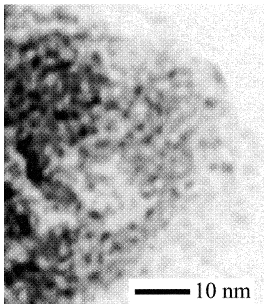
Fig. 6. TEM image of a tin sample prepared from templating electrolyte T1.
